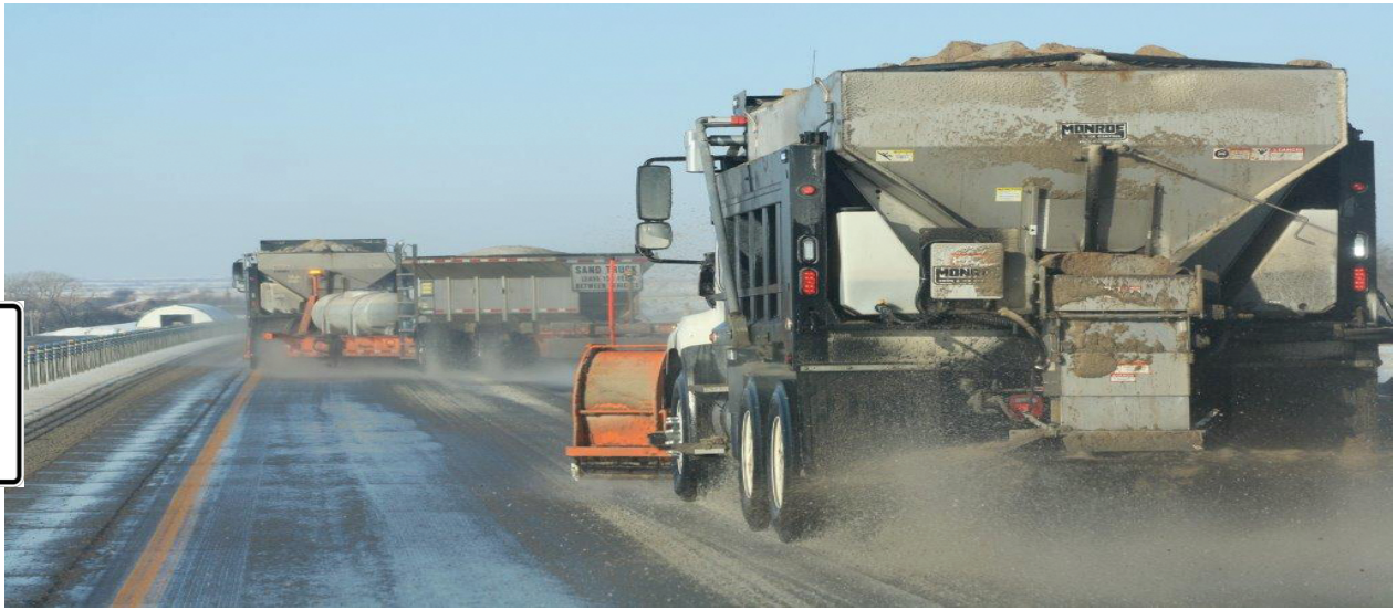
Cimarron Turnpike Wing plow and Tow plow
