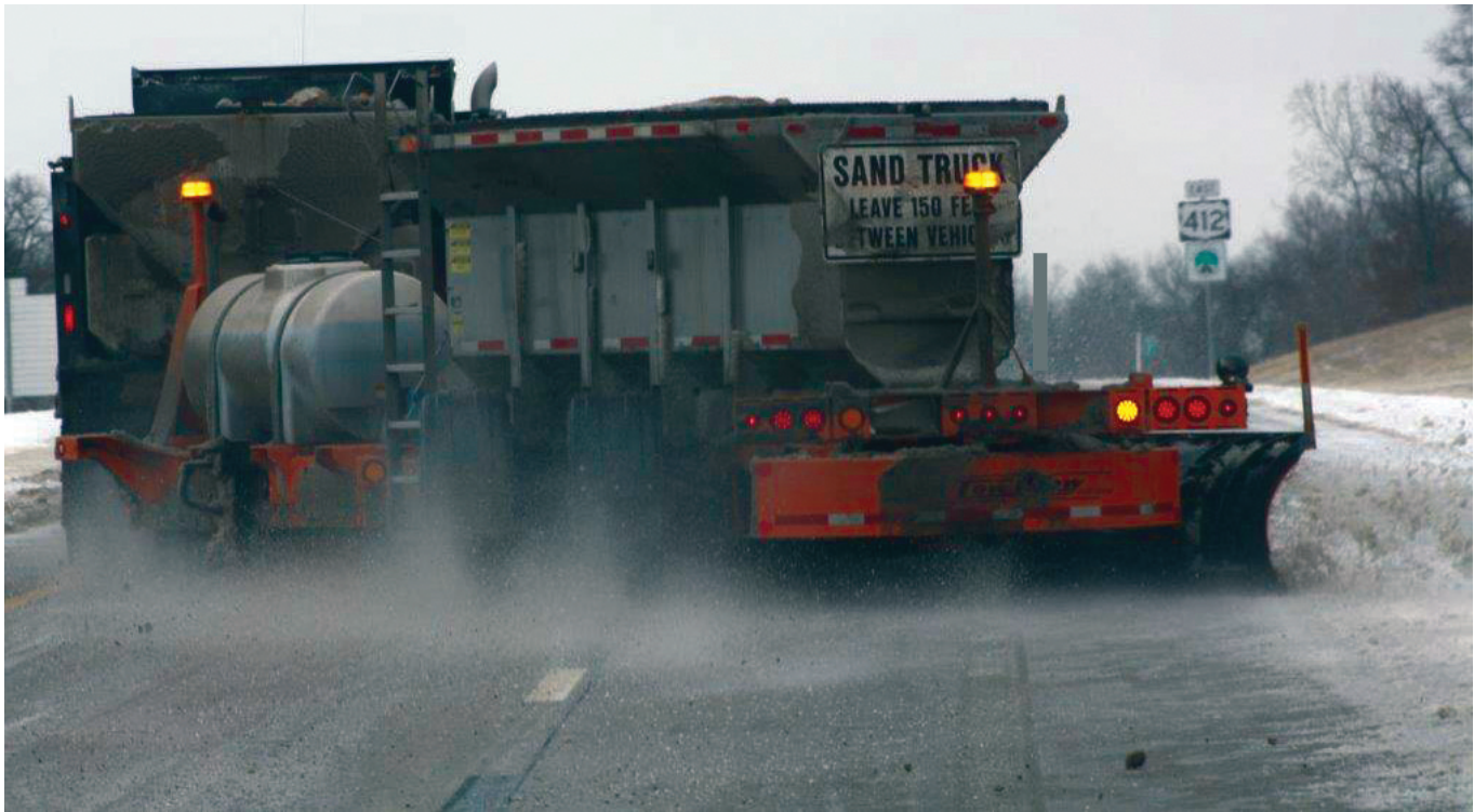
Cimarron Turnpike Wing plow and Tow plow
